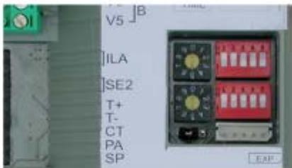
The dip-switches fitted in each device immediately associate addresses to individual users.
